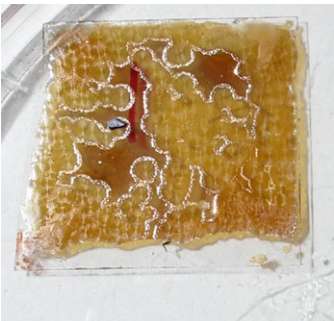
Left, I dissolved silver nitrate (AgNO 3 ) in polyethylene glycol diacrylate (PEG-DA), along with a crosslinking agent. I spun coat this solution onto 1" square glass slides. After deposition, the silver salt crystallized until the polymers was soldified by UV curing.
